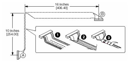
Figure 29: SCSI Cable Length Required
